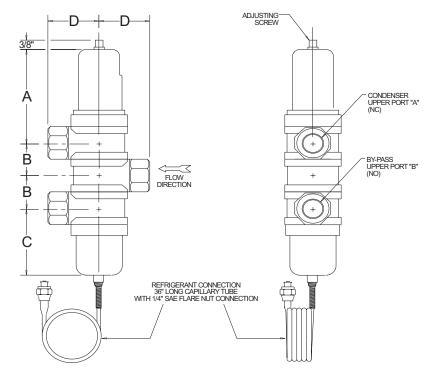
\*NOTE: Normally closed (NC) ports open on pressure increase, Normally open (NO) ports close on pressure increase.
