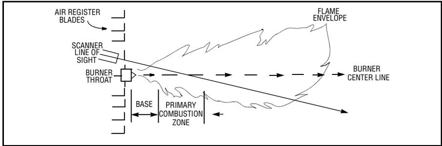
4. Consideration must be given to burner secondary air rotation, some burners have clockwise (CW) air rotation and others have counterclockwise (CCW) air rotation. If combustion air enters the furnace with a rotational movement of sufficient velocity to deflect the ignitor flame in the direction of rotation, position the scanner 10 to 30 degrees downstream of the ignitor as shown in Figure 5 and close to the periphery of the burner throat (See Figure 4).
