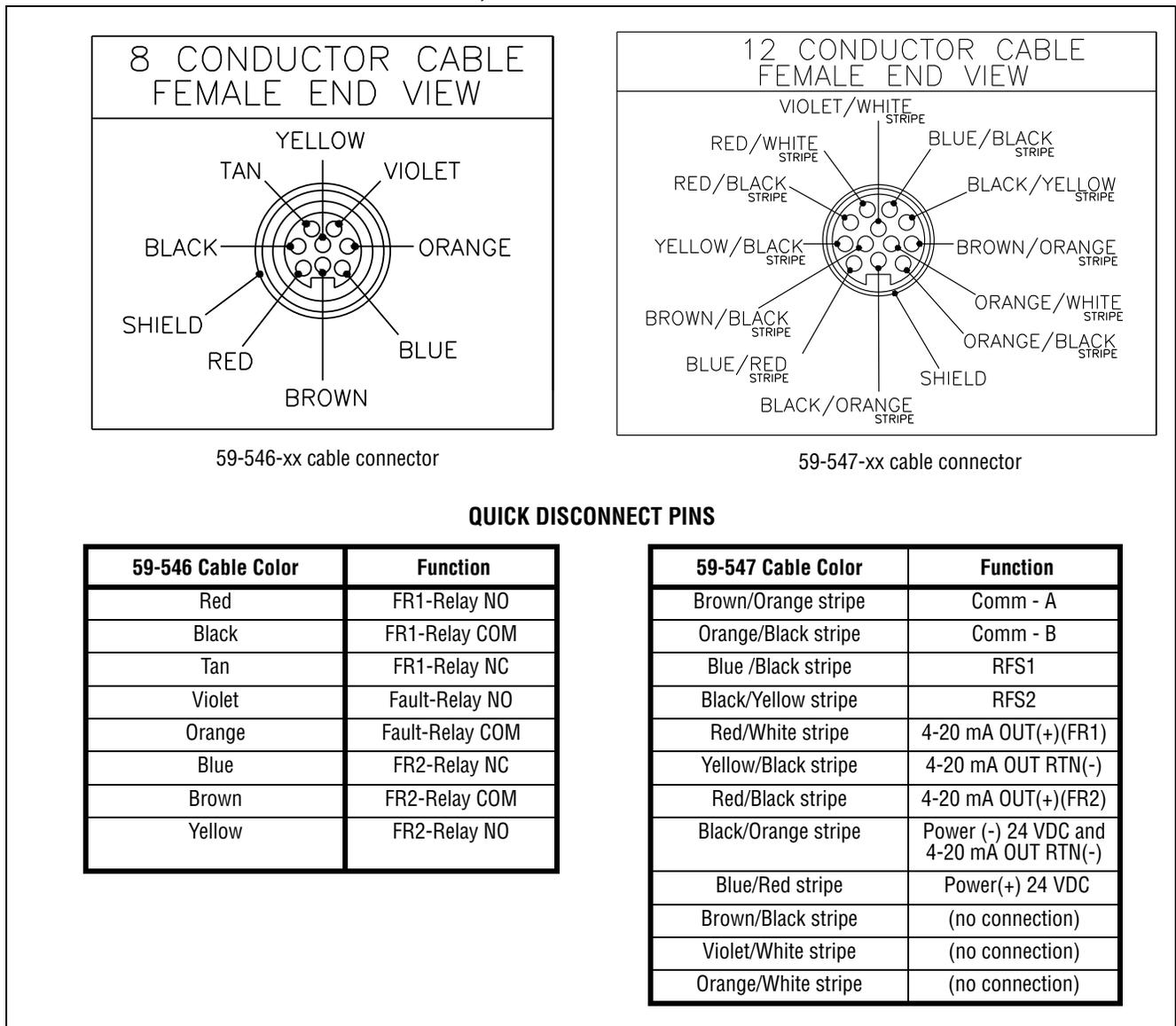
**FIGURE 16. WIRING FOR 95DSS3-1WOC, 95DSS3-1CEX, 95DSS3-1WICEX SCANNERS**
