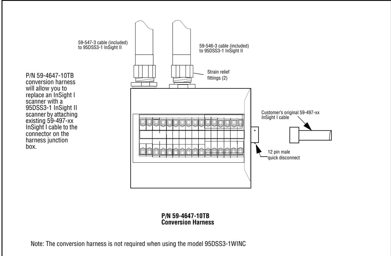
**FIGURE 20. WIRING DIAGRAM FOR P/N 59-4647-10TB CONVERSION HARNESS**
