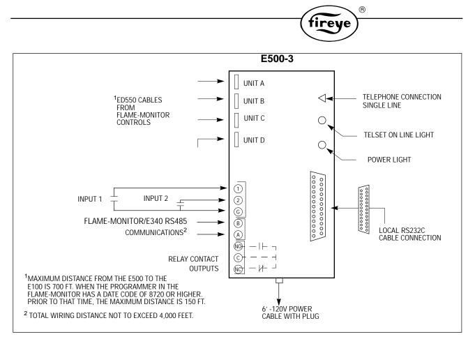
RS232C-style connections and cables are available at many computer stores. Minimum pin requirements for this cable are #'s 1, 2, 3, 7, 8, 20. Maximum Distance for Local RS232 C Cable:
