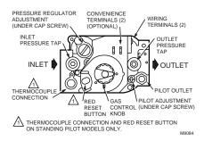
Fig. 1. Top view of VR8200 combination gas control.
