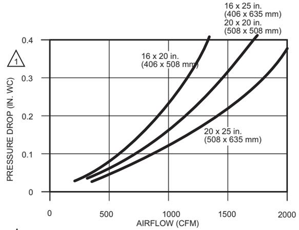
**1** WHEN FIRST INSTALLED. PRESSURE DROP INCREASES AS FILTER BECOMES LOADED. REPLACE FILTER WHEN PRESSURE DROP REACHES 0.5 IN. WC. (0.1 kPa).
