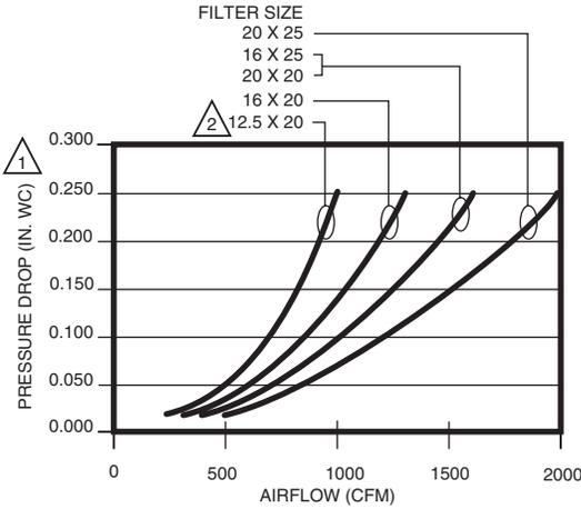
**1** WHEN FIRST INSTALLED. PRESSURE DROP INCREASES AS FILTER BECOMES LOADED. REPLACE FILTER WHEN PRESSURE DROP REACHES 0.5 IN. WC. (0.1 kPa).
