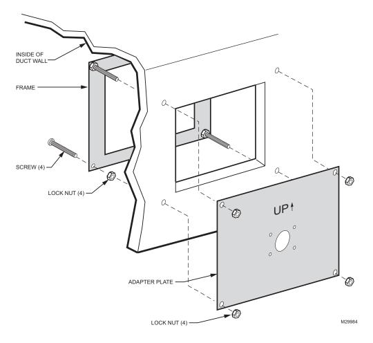
Fig. 1. Attaching the frame and adapter plate to the duct board.
