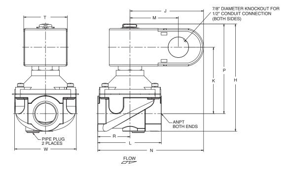
Must be mounted with solenoid vertical and upright or in a horizontal position.
