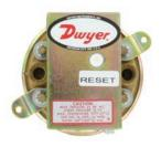
Manual reset Model 1900 MR includes special snap switch which latches on pressure increase above the setpoint. Switch must be manually reset after pressure drops below the setpoint. To order, change base model to 1900 and add MR suffix after range number. Example: 1900-10-MR. Available on -1, -5,-10 or -20 ranges only. Option is not UL, CSA or FM listed
