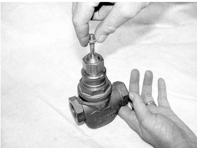
**STEP 1)** Assemble the supplied stem nut (E) to the valve stem, and thread at least 10 - 12 turns down onto the stem.
