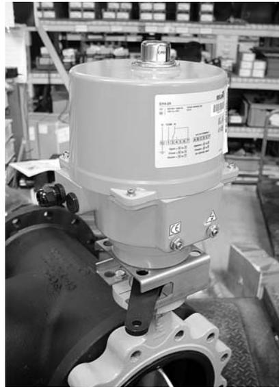
**Step 18)** When mechanical assembly is complete, the SY actuator and MASTER valve should be oriented as shown below. The actuator is in the OPEN position, and the valve disc is fully OPEN, and all bolts are tight.
