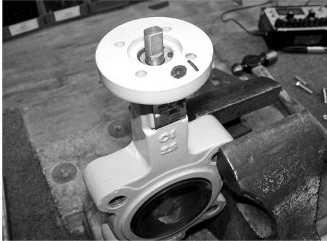
The valve should be stripped down to its basic form, as shown. Remove all other linkage components before starting the assembly sequence below. The linkage components have been designed to attach to the valve in this state, rather than to any existing hardware.
