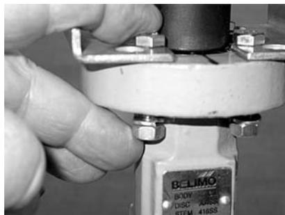
**Step 6)** Insert the four mounting bolts (B), lockwashers (C), and the hex nuts (D). Do NOT tighten at this time.
