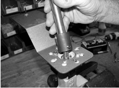
**Step 3)** Determine the position of the valve disc. Most manufacturers mark the TOP of the valve stem with a slot which indicates the disc angle. Slide the drive pin assembly, consisting of the drive shaft (E), the valve
