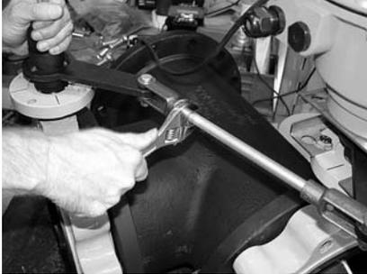
**Step 26)** Once the SLAVE valve has been determined to be in the correct position, lock the jam nut against one of the yoke ends to prevent any changes in the adjustments just completed.
