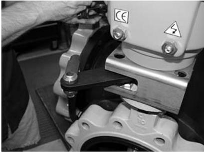
**Step 20)** With the MASTER valve in its fully OPEN position and the SLAVE valve in its fully CLOSED position, assemble the yoke and clevis pins onto the crank arms, pointing towards each other as shown.
