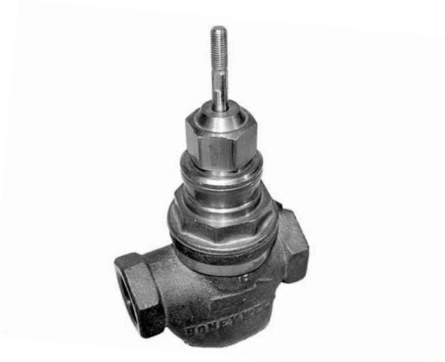
The valve should be stripped down to its basic form, as shown. Note that there are no threads on the bonnet. The packing nut is smaller than the diameter of the bonnet. There is a groove in the bonnet used to secure the retrofit collar to the valve.
