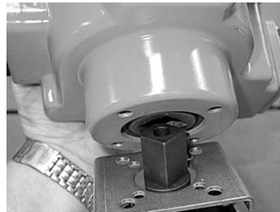
actuator with the square drive or keys in the coupling (C). The SY actuator will slide completely over the drive square and will rest ON the mounting bracket (A).
