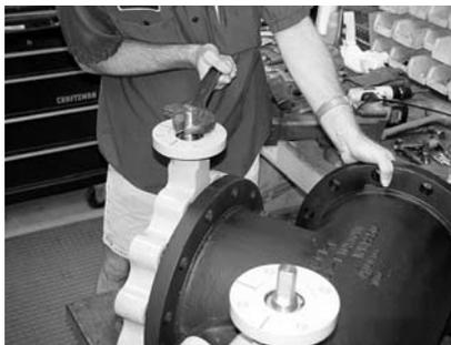
**Step 2)** Referring to the three configuration types on page 3 of the SY IOM, position the master and slave valve discs as instructed. For example, if you have a configuration code X20 tee assembly, you will OPEN the Master valve (M) and CLOSE the Slave valve (S).
