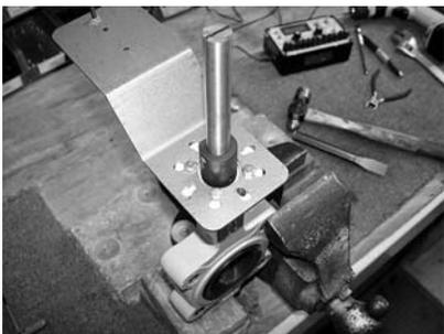
**Step 5)** Mark the TOP of the drive shaft to indicate the valve disc position. At this time, you should rotate the valve disc so that it is in the closed position. This will help facilitate proper attachment of the actuator.
