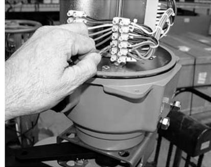
**Step 6)** Apply proper voltage to terminals 1 (Neutral) & 7 (Hot). Apply proper actuator voltage to terminals 1 (Neutral) & 4 (Hot) to drive the actuator CLOSED until the end-of-travel cam STOPS the actuator movement.
