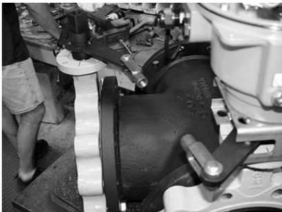
**Step 21)** Measure the distance between the inboard end of the yokes to determine the proper length of the connecting rod. It is important to make sure the MASTER and SLAVE valves are in their proper positions (OPEN and CLOSED, respectively) before
