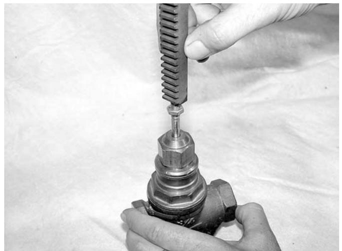
**STEP 2)** Attach the rack assembly (F), which may or may not include an extension or adapter, onto the valve stem. Thread the assembly as far down onto the valve stem as possible, until you contact the previously attached valve stem nut.
