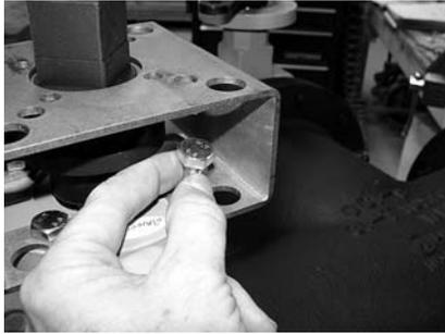
**Step 7)** Insert the four bolts and mount the bracket to the valve mounting flange. Attach the lock washers and nuts, but do NOT tighten at this time.
