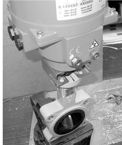
**Step 15)** When mechanical assembly is complete, the SY actuator and valve body should be oriented as shown below. The actuator is in the OPEN position, and the valve disc is fully OPEN. All bolts are tight, and electrical checkout is now possible.
