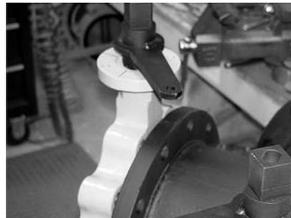
**Step 19)** The SLAVE valve is fully CLOSED with the crank arm oriented as shown.
