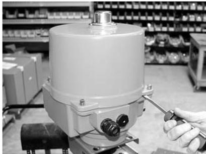
**Step 2)** Remove cover from the SY actuator. A flat blade screwdriver inserted carefully into the provided slot (as shown) will facilitate removal of the cover.
