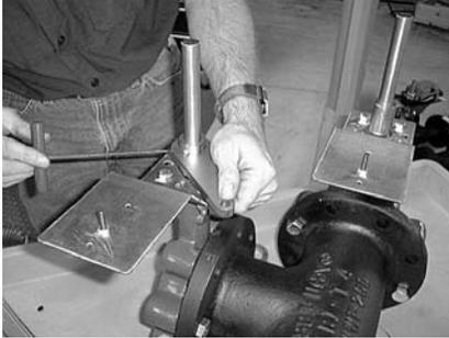
**Step 5)** Refer to the three configuration drawing types and position the crank arms (K) as instructed. Slide the crank arms over valve couplings (F), and position just below the top edge of the couplings. Tighten set screws (H) to affix the crank arms (K) to the couplings (F).
