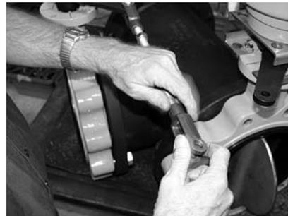
**Step 23)** Remove the MASTER valve yoke end and thread it onto the connecting rod. Adjust the distance between the yoke centers to match the hole in the MASTER valve crank arm.
