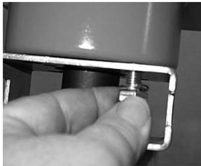
**Step 12)** Insert the four hex bolts (G) and lock washers (F) through the bracket and into the bottom of the SY actuator as shown. Do NOT tighten until all four sets have been installed. Slight twisting of the entire SY actuator will facilitate alignment of the bolts.
