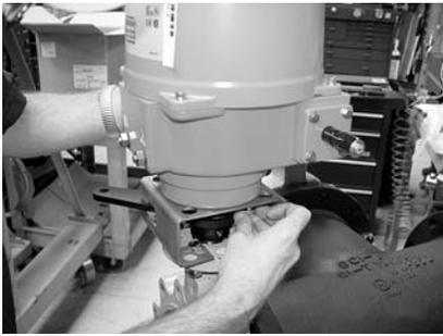
**Step 14)** Stand with the opening in the actuator bracket facing towards your LEFT. Hold the SY actuator with the handwheel on the RIGHT, and the EMT connectors to your LEFT. Align the square drive or keyway in the SY
