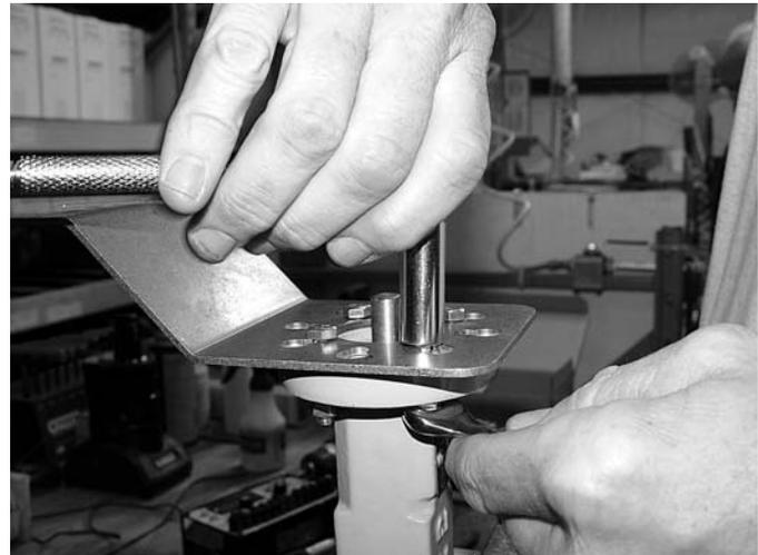
**Step 2)** Once all four bolts, lock washers and nuts have been assembled onto the valve body, tighten securely.
