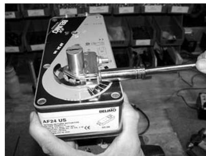
**Step 8)** For AF series actuators, release the pre-load on the spring before tightening the clamp nuts, as the valve disc has already been positioned at the fully closed position. For fail open requirements, pre-wind the AF spring to full open position before
