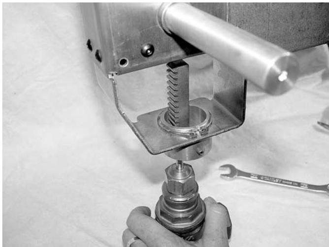
**STEP 4)** Slide the gearbox (A) assembly over the rack and down onto the valve bonnet nut. Note that the rack teeth must point TOWARDS the linkage drive shaft (B), and that the rack enters a small square hole in the bottom of the gearbox when aligned properly. It may be necessary to loosen the setscrew (G) in the linkage collar (C) before it will seat fully onto the valve bonnet.
