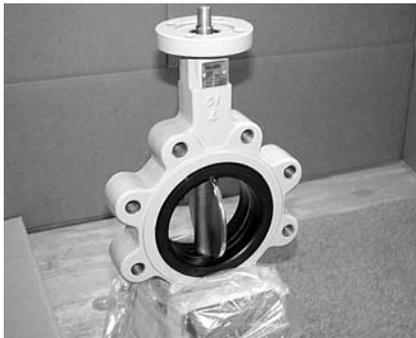
**Step 1)** The valve must be stripped down to its basic form. Remove all other linkage components before starting the assembly sequence below. The linkage components have been designed to attach to the existing valve flange rather than to any existing hardware.
