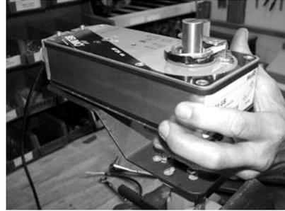
**Step 6)** Assemble the actuator to the linkage by sliding the actuator shaft clamp over the kit drive shaft (E). The actuator anti-rotation pin (I) should already be positioned in the correct hole for the actuator, but it can be moved to
