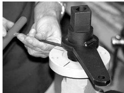
**Step 5)** Shown here is the SLAVE crank arm assembly being secured to the valve stem. Notice the markings on the valve top works indicating OPEN and CLOSED positions of the stem for later reference. Once set, crankarms may require spot
