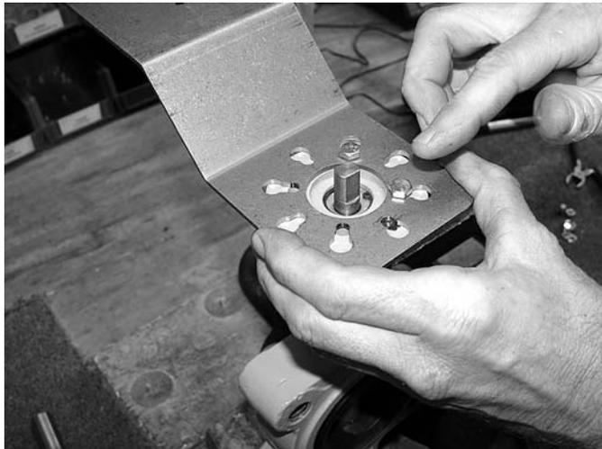
**Step 1)** Assemble the actuator mounting bracket (A) to the top of the valve actuator mounting pad using the supplied bolts (B), lock washers (C) and nuts (D). The bracket does NOT need to be oriented on the valve body in any particular position, however, the bracket should not come into contact with pipes, conduit or walls.
