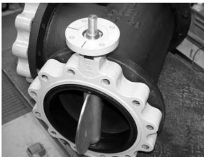
**Step 1)** Both valves must be stripped down to their basic form. Remove all other linkage components before starting the assembly sequence below. The linkage components have been designed to attach to the valves in their basic form state rather than to any existing hardware.
