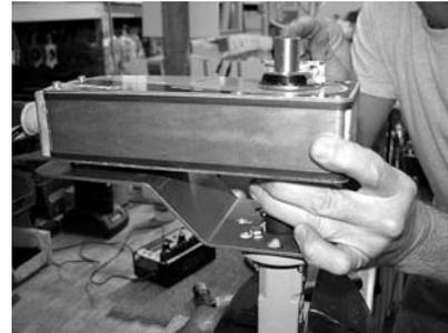
**Step 7)** Make sure the bottom of the actuator is PARALLEL to the mounting plate (A) when tightening the actuator clamp nuts. If this is not checked, it is possible that binding could cause erratic movement of the valve disc due to reduced torque transmission to the valve shaft.
