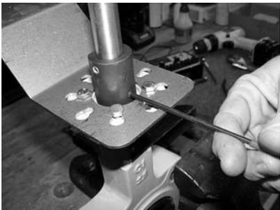
**Step 4)** Once the drive pin assembly has been seated onto the valve stem, tighten setscrew (H) to lock the assembly onto the valve shaft. The drive shaft (E) should be concentric and parallel with the valve shaft so there is no binding.
