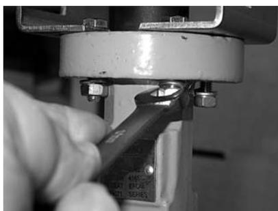
**Step 14)** Now tighten the four bracket bolts (B, C, D) assembled previously in step 6 .
