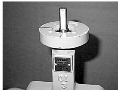
**Step 2)** The valve has either flats, a key slot, holes or a mark indicating the position of the disc with respect to the shaft. Usually, the flats, keys, holes and marks are PARALLEL to the valve disc. The photo at left shows the flattened shaft in the CLOSED position.
