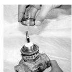
**STEP 2)** Be sure to retain all packing components which may come loose from the valve during the retrofit process.
