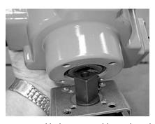
Step 9) Stand with the valve face (where the piping flange connects to the valve body) towards you. Hold the SY actuator with the handwheel on the RIGHT, and the EMT connectors to your LEFT. Align the square drive or keyway in the SY
