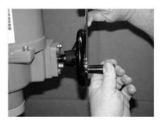
**Step 13)** Tighten the jam nut to prevent the hand knob from coming loose.
