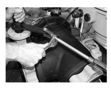
Step 26) Once the SLAVE valve has been determined to be in the correct position, lock the jam nut against one of the yoke ends to prevent any changes in the adjustments just completed.
