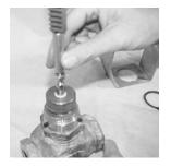
STEP 8) Attach the rack assembly (F), which may or may not include an extension or adapter. onto the valve stem. Thread the assembly as far down onto the valve stem as possible, until you contact the previously attached valve stem nut.
