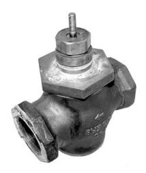
The valve should be stripped down to its basic form, as shown. The linkage components have been designed to attach to the valve in this state, rather than to any existing hardware. Note that there are no threads on the bonnet. The packing nut is smaller that the diameter of the bonnet. There is a groove in the bonnet used to secure the retrofit collar to the valve.
