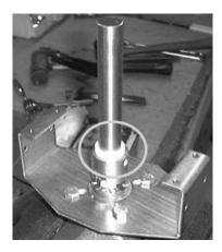
Step 4) Place the coupling shaft assembly onto the valve stem.
