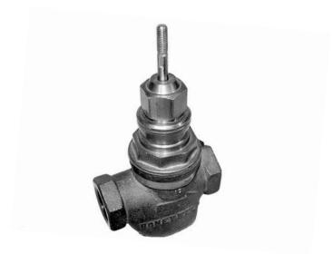
The valve should be stripped down to its basic form, as shown. Note that there are no threads on the bonnet. The packing nut is smaller that the diameter of the bonnet. There is a groove in the bonnet used to secure the retrofit collar to the valve.
