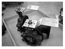
Step 2) Refer to the three configuration drawing types on pages 133 and 134 and position the valve discs as instructed. For example, if you have a Configuration Type A tee assembly, you will OPEN the master valve (A), and CLOSE the slave
