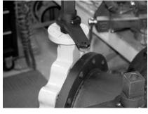
**Step 19)** The SLAVE valve is fully CLOSED with the crank arm oriented as shown.
