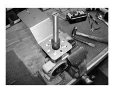
Step 5) Mark the TOP of the drive shaft to indicate the valve disc position. At this time, you should rotate the valve disc so that it is in the closed position. This will help facilitate proper attachment of the actuator.
