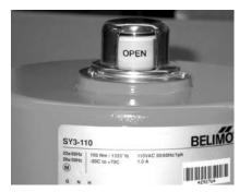
Step 7) The SY actuator is shipped in the OPEN position. Make sure the actuator is in the OPEN position before attaching to the valve/coupling assembly. The SY actuator turns counter clockwise (CCW) to the OPEN position, when viewed from ABOVE the actuator.
