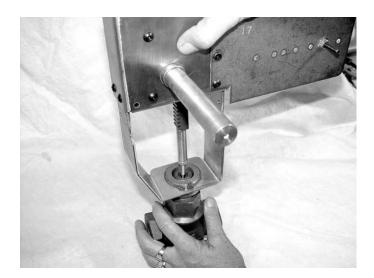
**STEP 4)** Slide the gearbox **(A)** assembly over the rack and down onto the valve bonnet nut. Note the the rack teeth must point TOWARDS the linkage drive shaft **(B)**, and that the rack enters a small square hole in the bottom of the gearbox when aligned properly.
