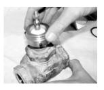
**STEP 5)** Assemble the supplied collar **(C)** to the valve bonnet. It may be necessary to loosen the three retaining setscrews **(G)**.
