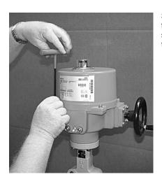
**Step 1)** Remove the four hex bolts securing the cover to the base casting.
