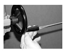
**Step 10)** Attach the hand knob to the hand wheel as shown below (if not already completed).
