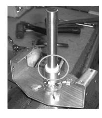
Step 4) Place the coupling shaft assembly onto the valve stem. Tap in place until coupling is fully seated on the valve stem. Put two or three (as needed) 3/4 inch nylon washers (P/N 44092) (circled in white) onto the shaft to make a snug fit.
