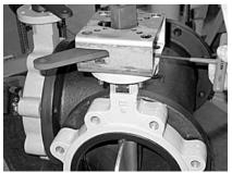
Step 4) Tighten the MASTER and SLAVE crank arm assemblies using the appropriate hex key wrench. Make sure the drive couplings are fully seated onto the valve stems BEFORE tightening the set screws.
