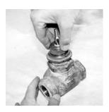
**STEP 1)** Remove system pressure from the valve. Remove the external packing nut.
