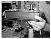
Step 7) Make sure the bottom of the actuator is PARALLEL to the mounting plate (A) when tightening the actuator clamp nuts. If this is not checked, it is possible that binding could cause erratic movement of the valve
