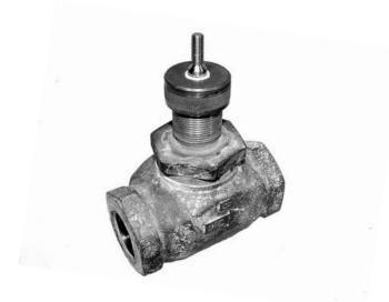
The valve should be stripped down to its basic form, as shown. Note that many pneumatically operated valves have hardware that must be removed from the threaded bonnet area before measurements can be taken.
