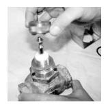
STEP 6) Reattach the packing nut removed in step 1. Be sure to replace all packing materials that may have come loose during the retrofit process.
