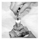
STEP 7) Assemble the supplied stem nut (E) to the valve stem, and thread at least 10 - 12 turns down onto the stem.
