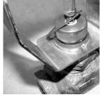
STEP 11) After the linkage has been seated on the collar, turn the linkage until the key in the collar (C), lines up with and engages the key in the base of the linkage.
