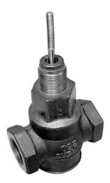
The valve should be stripped down to its basic form, as shown. The linkage components have been designed to attach to the valve in this state, rather than to any existing hardware. Note that this style valve has an internal packing nut, which does NOT interfere with the bonnet threads.
