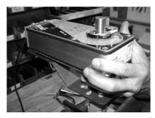
Step 6) Assemble the actuator to the linkage by sliding the actuator shaft clamp over the kit drive shaft (E). The actuator anti-rotation pin (I) should already be positioned in the correct hole for the actuator, but it can be moved to
