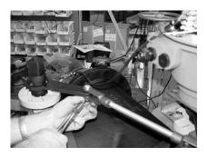
**Step 27)** Insert two cotter keys into the two clevis pins.
