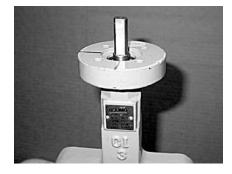
Step 2) The valve has either flats, a key slot, holes or a mark indicating the position of the disc with respect to the shaft. Usually, the flats, keys, holes and marks are PARALLEL to the valve disc. The photo at left shows the flatted shaft in the CLOSED position.
