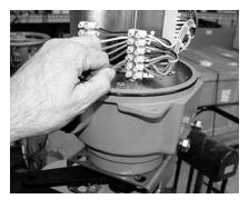
Step 6) Apply proper voltage to terminals 1 (Neutral) & 7 (Hot). Apply proper actuator voltage to terminals 1 (Neutral) & 4 (Hot) to drive the actuator CLOSED until the end-of-travel cam STOPS the actuator movement.
