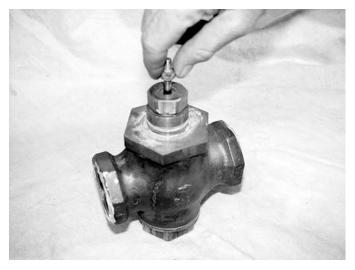
STEP 1) Assemble the supplied stem nut (E) to the valve stem, and thread at least 10 - 12 turns down onto the stem.
