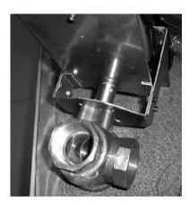
Step 11) For 3-way ball valves: The 3-way ball valve assembly is completed the same way with AF, GM, single, actuators.
