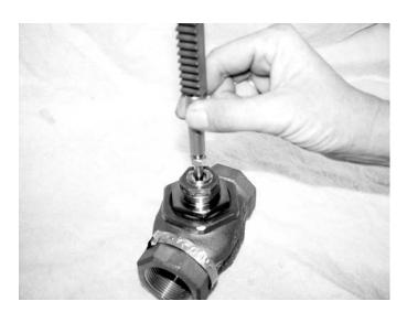
**STEP 2)** Attach the rack assembly **(F)**, which may or may not include an extension or adapter, onto the valve stem. Thread the assembly as far down onto the valve stem as possible, until you contact the previously attached valve stem nut.
