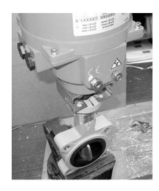
Step 15) When mechanical assembly is complete, the SY actuator and valve body should be oriented as shown below. The actuator is in the OPEN position, and the valve disc is fully OPEN. All bolts are tight, and electrical checkout is now possible.
