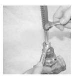
STEP 9) Use a 1/2" open end wrench, and an additional open end wrench sized to match the valve stem nut (E), to tighten the rack assembly (F) to the valve stem. Use the 1/2" open end wrench to attach to the smooth back side of the rack, opposite the teeth. This will prevent damage to the rack teeth during the tightening sequence.
