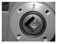
Step 8) Verify that the SY actuator is in the OPEN position also by looking at the bottom of the actuator. There is a dimple mark punched in the output shaft which will align with the "1" mark when the actuator is in the OPEN position.
