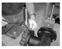
Step 5) Refer to the three configuration drawing types and position the crank arms (K) as instructed. Slide the crank arms over valve couplings (F), and position just below the top edge of the couplings. Tighten set screws (H) to affix the crank arms (K) to the couplings (F).
