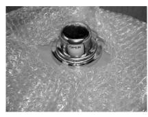
Step 10) Although the SY actuator ships from the factory IN the OPEN position, make sure the actuator is in the OPEN position before attaching to the valve/coupling assembly. The SY actuator turns counter clockwise (CCW) to the OPEN
