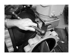
Step 24) Insert the clevis pin into the master crank arm.
