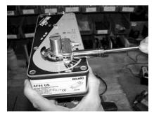
Step 8) For AF series actuators, release the pre-load on the spring before tightening the clamp nuts, as the valve disc has already been positioned at the fully closed position. For fail open requirements, pre-wind the AF spring to full open position before
