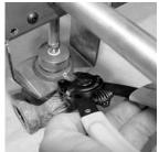
STEP 12) Attach the collar retaining ring (D) onto the collar, and press securely in place into the machined groove in the collar. You should hear a "snap" when the ring is fully seated.
