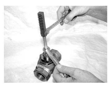
**STEP 3)** Use a 1/2" open end wrench, and an additional open end wrench sized to match the valve stem nut **(E)**, to tighten the rack assembly **(F)** to the valve stem. Use the 1/2" open end wrench to attach to the smooth back side of the rack, opposite the teeth. This will prevent damage to the rack teeth during the tightening sequence.
