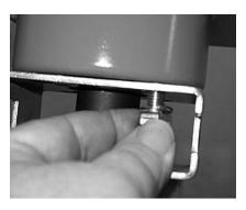
Step 15) Insert the four hex bolts (G) and lock washers (F) through the bracket and into the bottom of the SY actuator as shown. Do NOT tighten until all four sets have been installed. Slight twisting of the entire SY actuator will facilitate alignment of the bolts.
