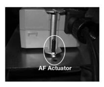
**Step 10)** Slide actuator down over the shaft and onto the tail pin.
