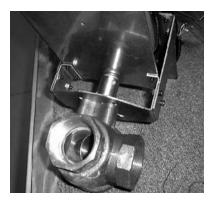
Step 14) 3-way ball valves: (FIG.BV-13) The 3-way ball valve assembly is completed the same way with dual actuators.
