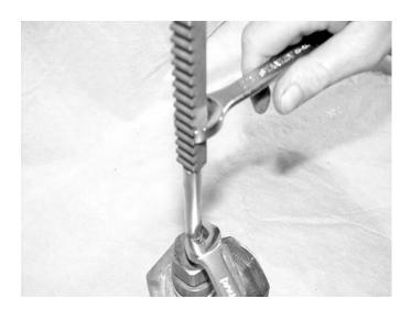
**STEP 3)** Use a 1/2" open end wrench, and an additional open end wrench sized to match the valve stem nut **(E)**, to tighten the rack assembly **(F)** to the valve stem. Use the 1/2" open end wrench to attach to the smooth back side of the rack, opposite the teeth. This will prevent damage to the rack teeth during the tightening sequence.
