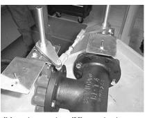
Step 7) The connecting rod (P) is supplied long enough to meet all configuration types, and will have to be modified in the field to properly fit your assembly. Connecting rod (P) is furnished with jamb nut (O), yoke (N), clevis pin
