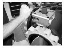
Step 8) To facilitate the insertion of the mounting bolts, it may be necessary to move the valve disc, and therefore the crank arm, to gain access to the mounting holes.
