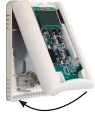
8. Use the switch to select voltage or current output. For CWL model, see Configuration section on page 4.
