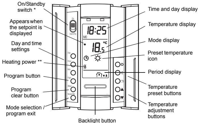
\* Set the switch to Standby to cut power to the heater. This will not affect the time and temperature settings.
