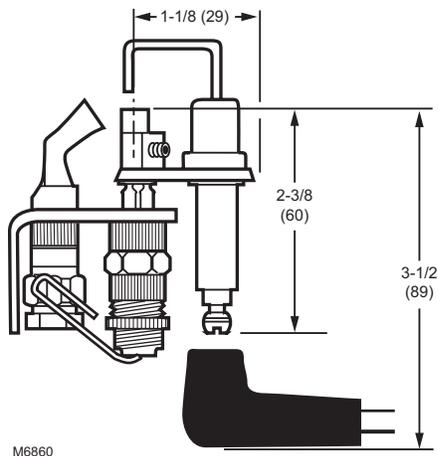
Fig. 5. 392431 Igniter-sensor mounting dimensions in inches. (mm).
