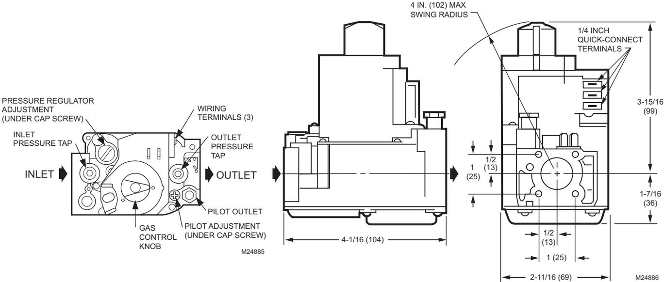
Fig. 3. VR8304M mounting dimensions in inches (mm).
