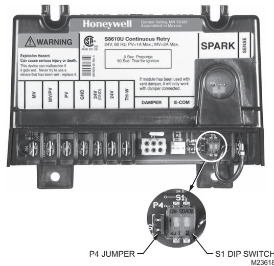
Fig. 18. DIP switch (S1) and jumper (P4) location.
