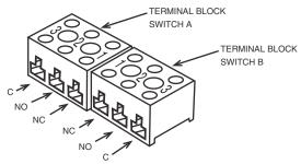
es mounted together in a bracket. Switches are calibrated to have simultaneous operation within 1% of range either on increasing or decreasing pressure but not in both directions. Wire directly to the front and rear switch according to circuit requirements. Leads are provided on rear switch color coded as follows:
