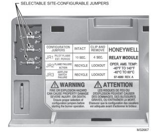
Fig. 15. Selectable site-configurable jumpers (RM7895 shown).
