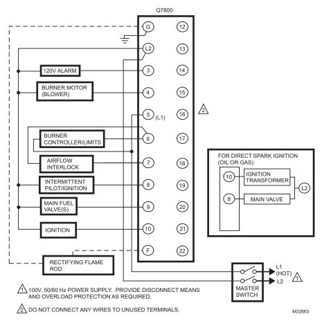
Fig. 6. Wiring the RM7895E, F Relay Module.
