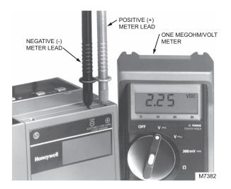
Fig. 16. Flame signal measurement.
