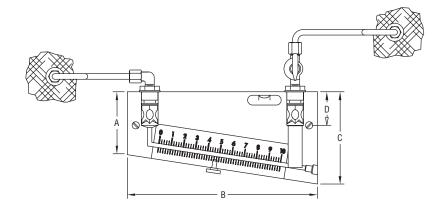
**Note:** The drawing above shows standard connection at left and three-way vent valve at right. If the optional vent valves are preferred, please note that two are required.
