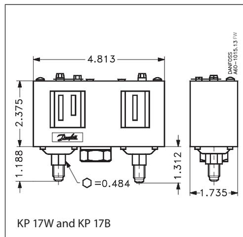
Capillary tube connection
