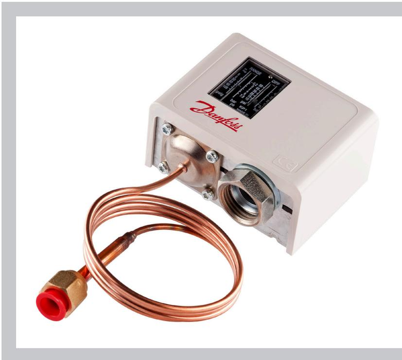
The KP pressure switches can be used as safety switches against too low a suction pressure and/or too high a discharge pressure in refrigeration and air conditioning systems. They can also be used to start/stop compressors and fans for air-cooled condensers.
