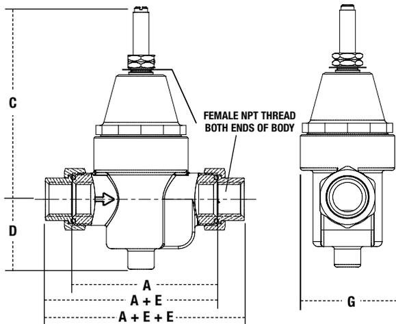
ABOVE VALVE SHOWN WITH SINGLE NPT UNION CONNECTION ON INLET
