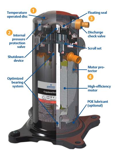
Copeland Scroll compressors feature a variety of internal safety controls, designed to ensure proper actuation of the internal line-break motor protection. These safety features include:
