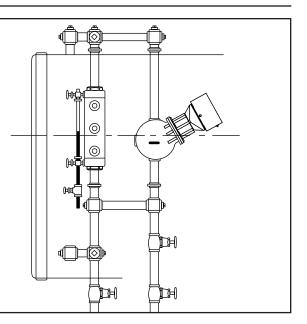
When the water level rises to the level of the top probe, the pump relay will be de-activated. Depending on the application, this will either turn off the pump or close a valve.
