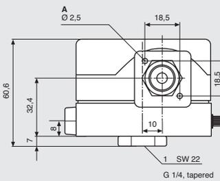
Pressure connection (+)  $\varnothing 4.6$  can only be used as test nipple. Pressure connection only possible using G 1/4.
