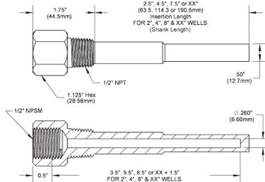
**Fig 8:** Machined Bar Stock Thermowell
