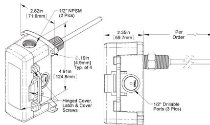
**Fig 2:** Double Threaded Immersion Sensor in a BAPI-Box 2 (BB2) Enclosure
