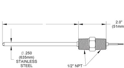
**Fig 7:** Double Threaded Stainless Steel Immersion Probe Only
