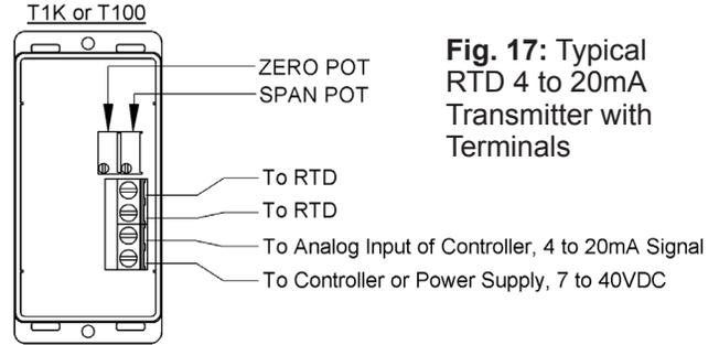
**Fig. 17:** Typical RTD 4 to 20mA Transmitter with Terminals
