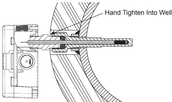
Fig 12: Typical Sensor Inserted
