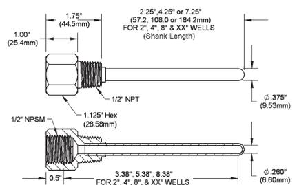
**Fig 9:** Two Part Welded Thermowell
