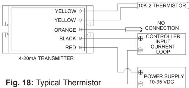
**Fig. 18:** Typical Thermistor 4 to 20mA Transmitter
