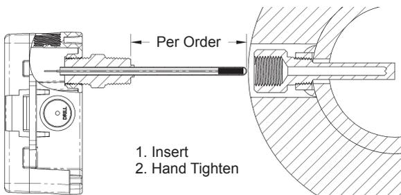
Fig 14: BAPI-Box 2 (BB2) Model Before Insertion
