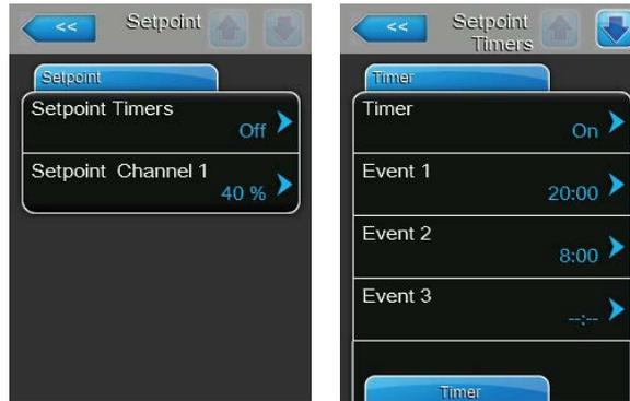
Activate the timer function (Setpoint Timers: "On"). If the setpoint timer is activated, up to eight switching points (Event 1... Event 8) with different humidity setpoints can be defined. Each switching point is defined by a weekday or weekday range, the switching time and the humidity setpoint in %rh.
