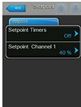
Let the timer function deactivated (Setpoint Timers: "**Off**") or deactivate the timer function if necessary. Then, set the desired humidity setpoint value in %rF via the "Setpoint Channel 1" parameter (Factory setting: **40 %rh**, Setting range: **5...95 %rh**).
