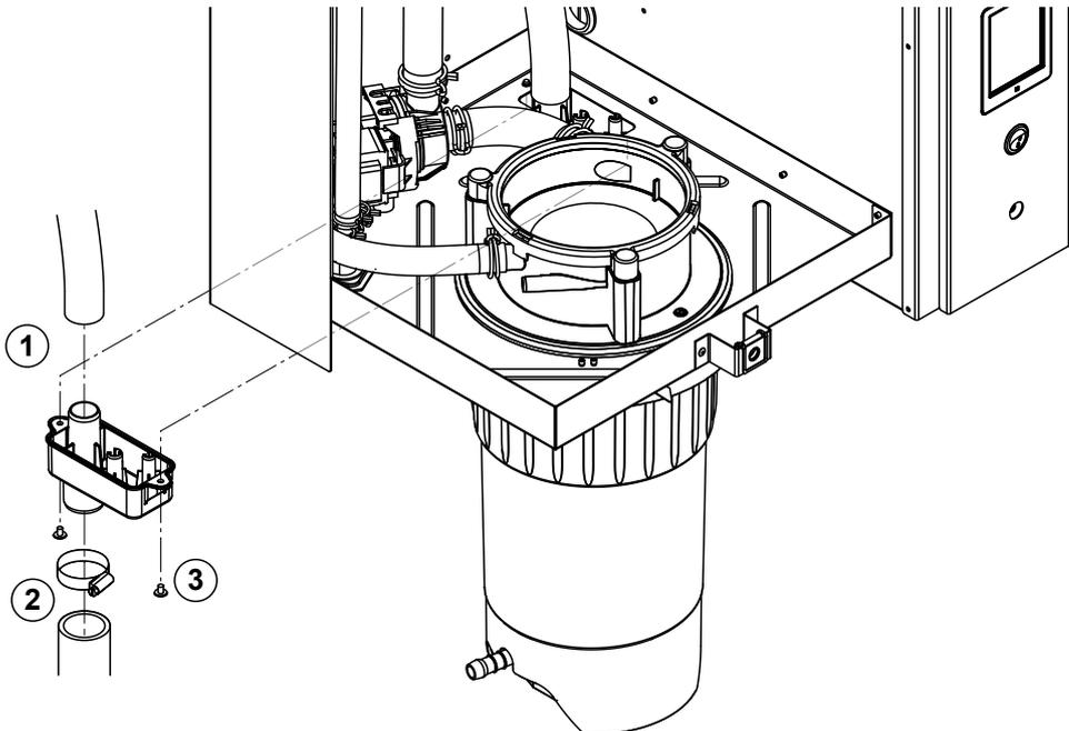
1. Remove drain hose from the connector on the drain cup.
