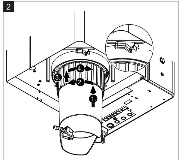
1. Insert the strainer insert into the corresponding receptacle inside the scale collector tank and press it down until it locks. Then, attach O-ring and Snap ring to the locking ring of the scale collector tank.
