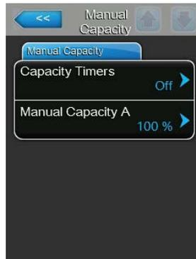
Let the timer function deactivated (Capacity Timers: "**Off**") or deactivate the timer function if necessary. Then, set the desired capacity limitation of the steam humidifier in % of the maximum capacity via the "Manual Capacity A" parameter (Factory setting: **100 %**, Setting range: **20 ... 100 %**).
