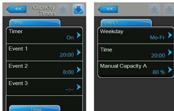
Activate the timer function (Capacity Timers: "**On**"). If the capacity timer is activated, up to eight switching points (Event 1... Event 8) with different capacity limits can be defined. Each switching point is defined by a weekday or weekday range, the switching time and the capacity limitation in % of the maximum capacity.
