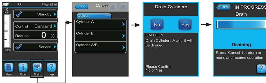
1. Press on the **<Drain>** button in the standard operating display. The "Manual" submenu appears.
