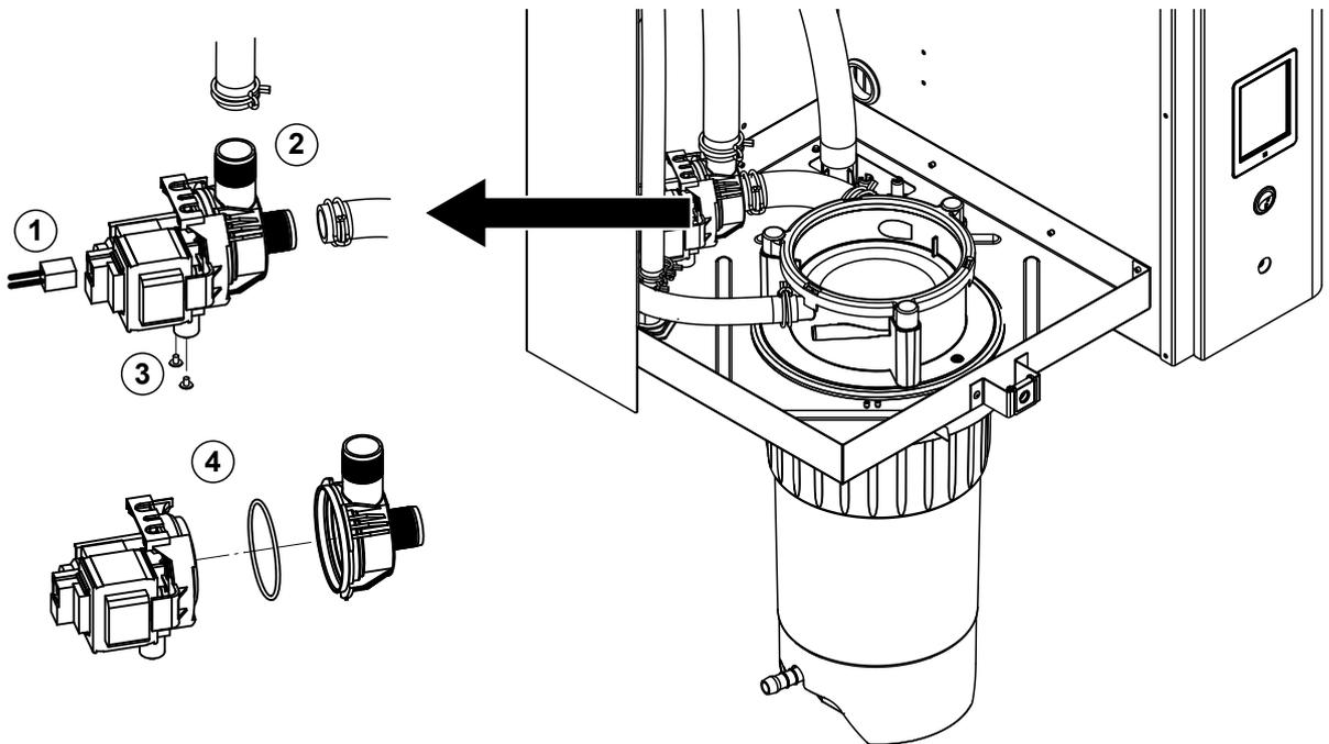
1. Detach electric cables (polarity of the cables must not be observed).
