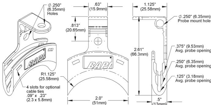
**Fig. 7: Flexible Probe Bracket (BA/FPB) (Order Separately)**
