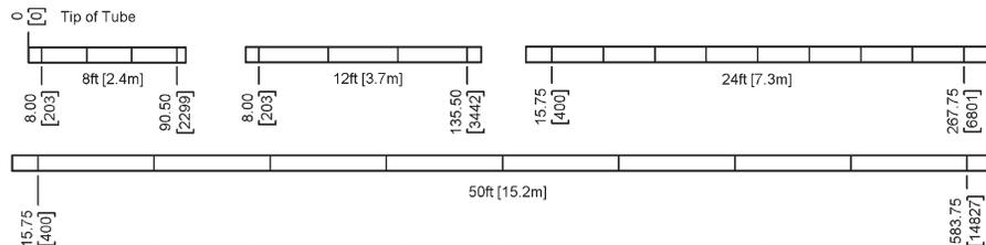
**Fig. 6: Thermistor Sensor Element Location in Probes**
