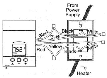
Attach wires per diagram above.
