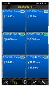
**Dashboard** - Location where up to 6 probes can be displayed simultaneously with their current readings.
