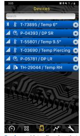
**Devices** - Lists all probes that are in communication with the app. Select probes to view live data or logs to graph or share.
