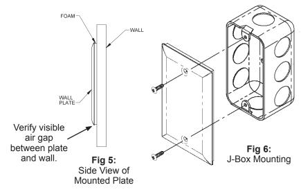
Note: Louvered wall plates require a mounting adapter bracket for J-Box mounting. The bracket is not shown in the diagram above but is included with any louvered wall plates ordered from BAPI.
