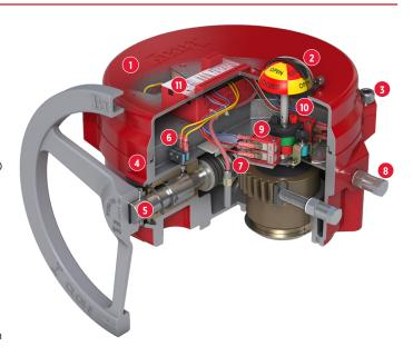
10 Limit Switch CAMs: Bray's patented CAM design includes standard green (open) and red (close) CAMs which are adjustable with finger touch or screwdriver. No additional tools necessary. Standard factory setting allows 90° travel between open and close positions.
