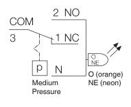
**GMH (Operating state shown) As pressure rises**, 2 NO closes, 1 NC opens, and Neon light ON (fault), switch trips and locks out.
