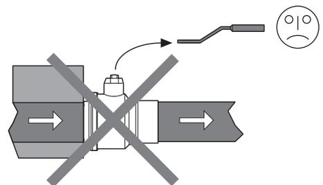
**!** Never permanently remove the handle from the ball valve.
