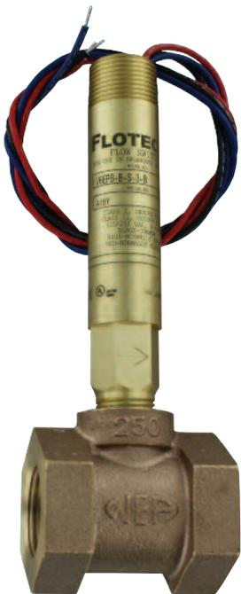
The Series V6 FLOTECT® Flow Switch is an inexpensive, explosion-proof flow switch for use on air, water or other compatible gases and liquids. Three configurations are available - 1. Factory installed in a tee. 2. With a trimmable vane for field adjustment and installation in a suitable tee. 3. Low flow models with an integral tee and adjustable valve. All are available with an optional enclosure which is UL and CSA listed, or Directive 94/9/EC (ATEX) compliant for
