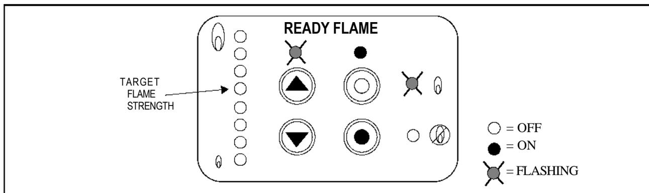
The Flame Strength should BRIEFLY GO BELOW 6 LEDs. If the LEDs stay at 7 or above, add orifices to minimize the signal (see page 29). If the signal strength does not drop below 6 LEDs, then decrease the size of the orifice. This may require some testing to determine the correct size.
