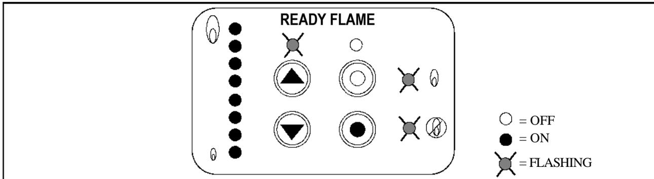
Keeping the target flame button depressed, use the flame strength LEDs to adjust the scanner “aim” to get maximum signal (1 LED is the lowest, 8 LEDs are the highest). Look for 3 to 4 LEDs as a minimum.
