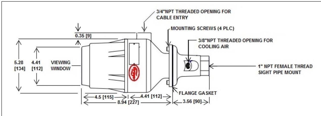
All models of the Phoenix 85UVF1/IRF1-1CEX and 85UVF1-1CEX-K3 flame scanners are housed within an ATEX approved housing for application in Ex II 2 G/D hazardous rated environment. In addition the ATEX housing is designed to meet the requirements of IP66 (NEMA 4X).
