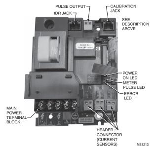
Fig. 16. Hardware Functions.
