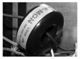
Fig. 6. Solid Core Sensor Assembly.
