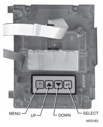
Fig. 17. Hardware Functions.
