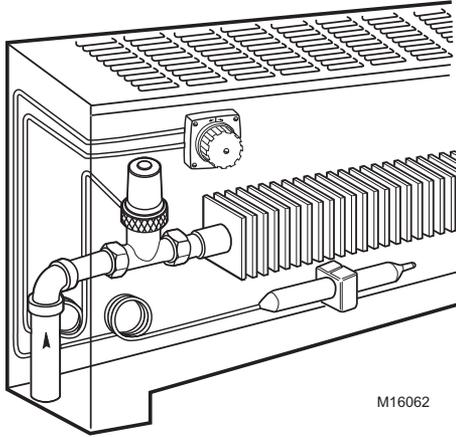
**Fig. 1. Mounting T100C on an enclosure shell.**
