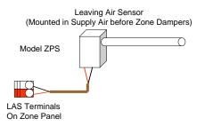
NOTE: If the ZPS is not used, the NO SENSOR jumper located just above the LAT terminals must be on the pins.
