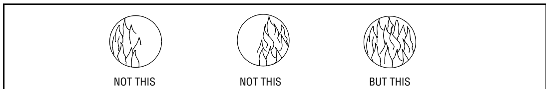
FIGURE 6. FLAME MUST COMPLETELY COVER SIGHT OPENING
