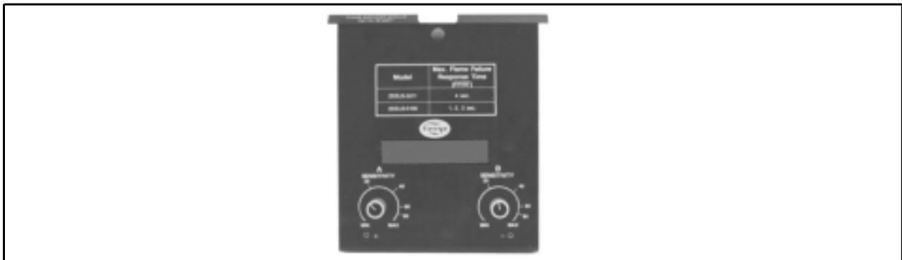
Each sensitivity control is adjustable for regulating the signal level in excess of the Flame Relay threshold. Turning the sensitivity in the clockwise direction amplifies the flame signal such that each graduation yields a reading twice that of the preceding.
