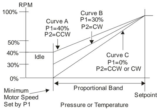
**Figure 12: Standard Input Mode**
