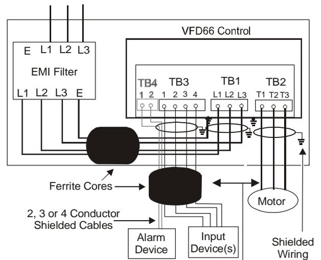
Separate input and output cables. Do not run input cables alongside output cables. Do not bundle input and output cables together.
