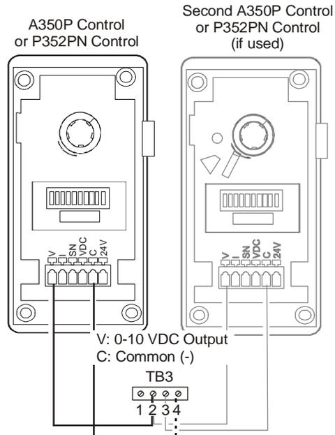
**Figure 6: Wiring A350P Controls or P352PN Controls to VFD66 Terminal Block 3**
