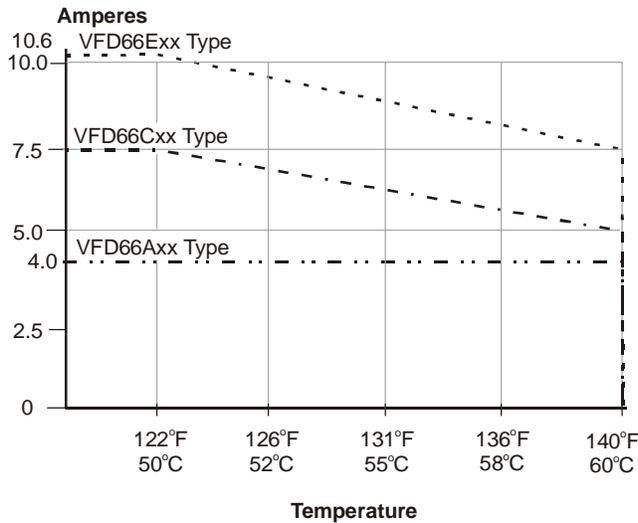
**Figure 10: 208/230 VAC Temperature De-Rating**
