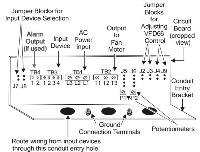
**Figure 3: Jumper Block, Terminal Block, and Potentiometer Locations**
