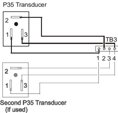
**Figure 4: Wiring P35 Transducers to VFD66 Terminal Block 3**
