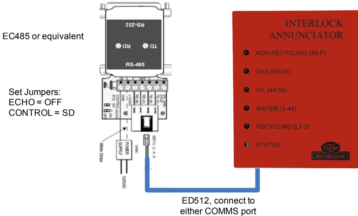
4. Plug one end of the ED512-2, -4 or -8 cable into the RJ12 jack on the EC485 and the other end into either of the RJ12 jacks located on the underside of the YZ300 Interlock Annunciator.
