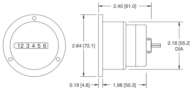
Mounting holes: For #4 screws on 2.44" [62.0] B.C.
